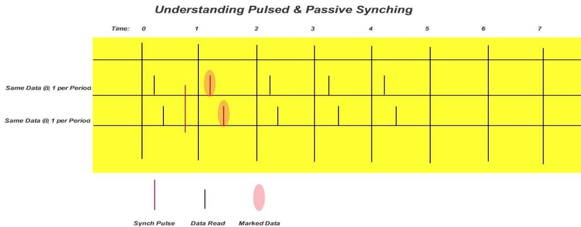
This diagram shows how the data would be aligned if the pulse occurred between the two readings. It demonstrates that marked data could be nearly one time period apart.
