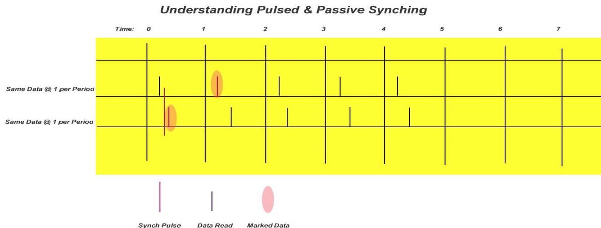
This diagram demonstrates an example of two data streams collected at different measurement rates. In the Slow Data stream, 1 sample is collected per period while the Fast Data is 2 samples per period.
