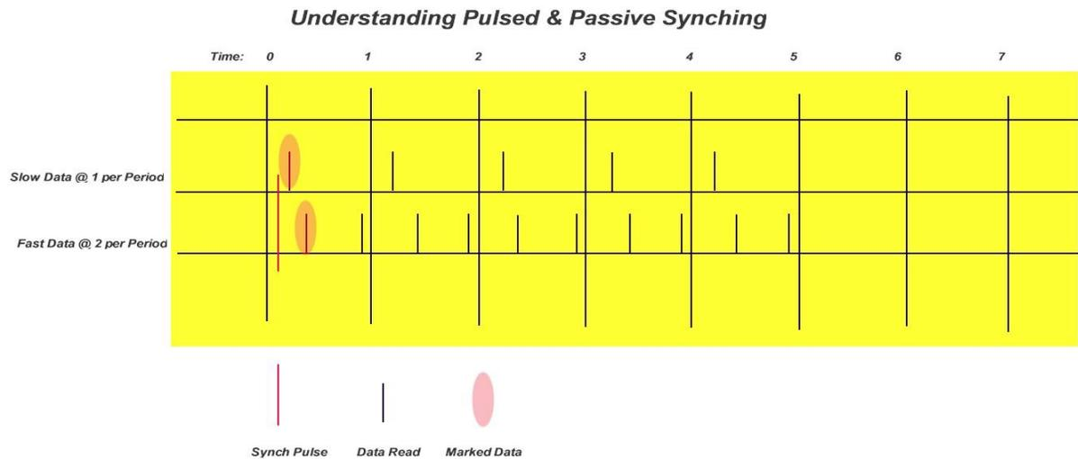
This diagram demonstrates an example where the event mark occurs between two readings with the separation in real time being almost a whole period.
