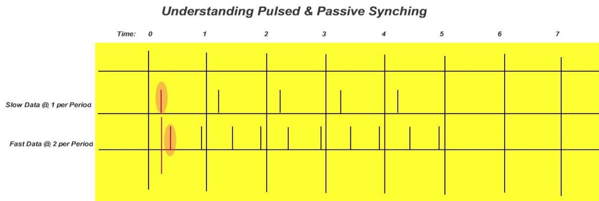
In this example, the Fast device is generating the signal and it demonstrates that the signals could be almost one period apart in real time
