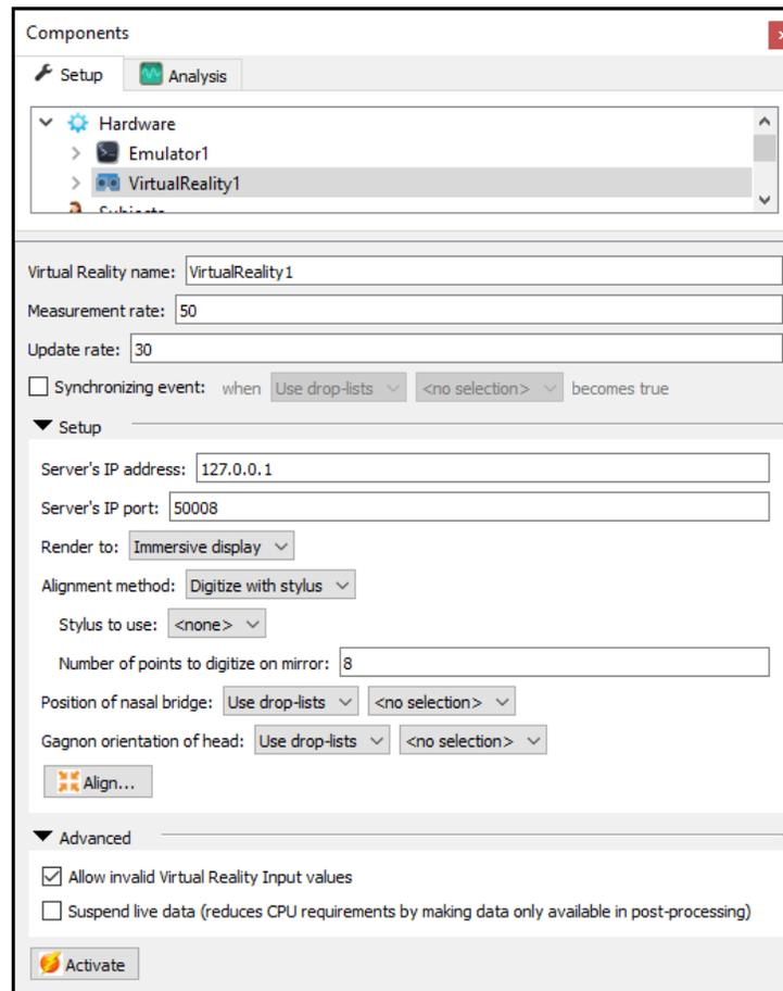
Enable the input of invalid values using the check box. Finally, select the medium for which the VR will be rendered to, either immersive display, Tobii HMD or standard HMD.
