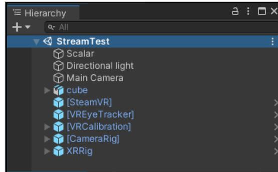
There is an item from the hierarchy that should be removed based on whether an HMD is used and it is desired to use the head compensation form the HMD or not. If the head compensation is desired, the [CameraRig] should be deleted. If no head compensation is desired, the XRRig should be deleted.
