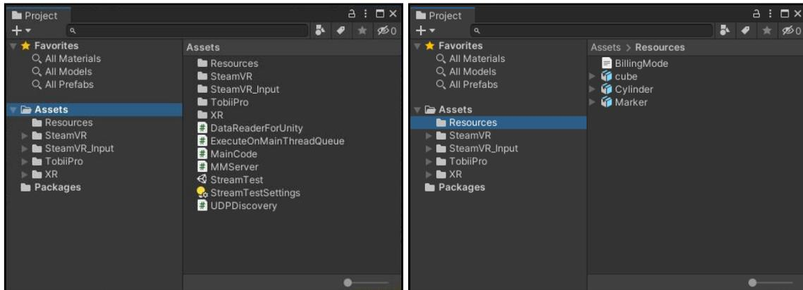
The Assets folder is where the 2 main scripts are located. The MainCode script is the base code for your Unity Project. This is where the Virtual Reality Inputs and Outputs that were discussed previously would be specified. The MMServer script is the script that communicates with The MotionMonitor xGen and where the Virtual Reality Objects and Biofeedback Cursors and Targets get automatically added to the Unity Project.
