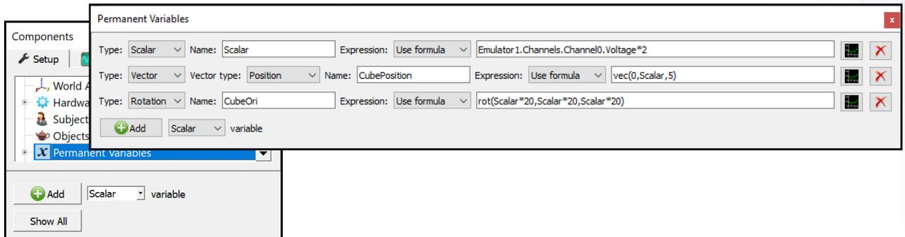
**Scalar** - This is the scalar variable that's being used for the "Scalar" Virtual Reality Input.
