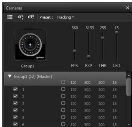
Depending on the camera model, there might also be a setting for Illumination Type under the camera settings. Strobed illumination is optimal for most standard data collection environments, while continuous is ideal for volumes where there may be interference from other IR devices.
