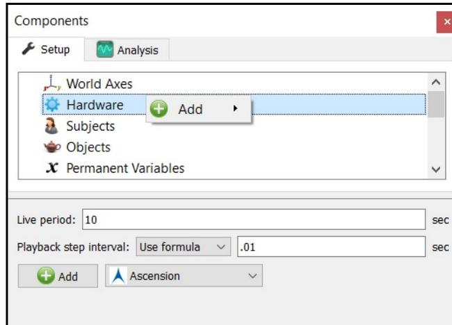
2. Click on the Ascension device to bring up the Ascension parameters panel. Specify the name and transmitter type, based on the transmitter type used, either standard range transmitter (36" or 72") or wide area transmitter (144" or 288"). Set the Report rate (valid settings include integers between 3-10, the default rate is 3) and Measurement rate (20-250 frames/sec).
