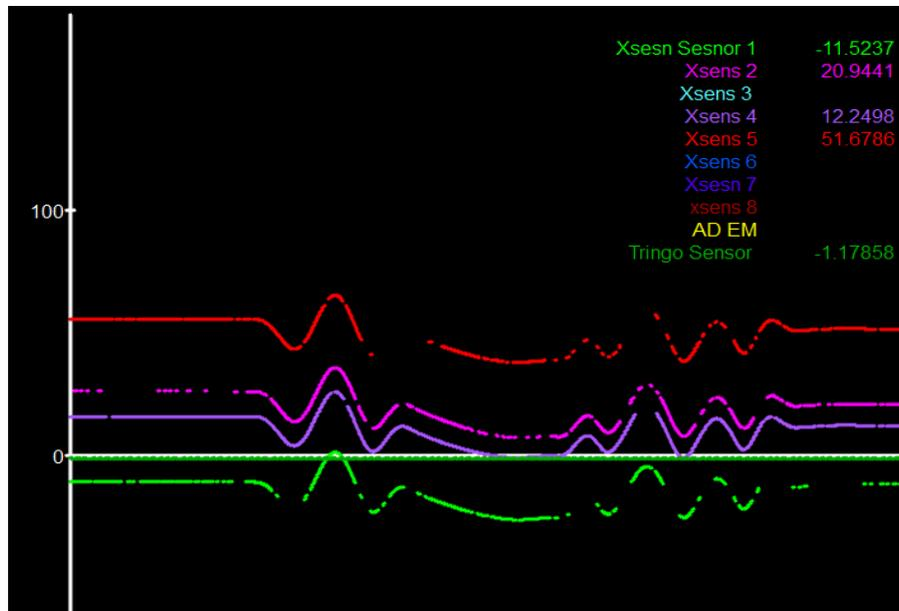
Wireless communication is subject to change in different environments. Radio channel selections may have to be changed if a system is used portably and data is collected in different spaces. It is recommended that channels are tested for each environment to determine which allow for the least amount of drop outs.
