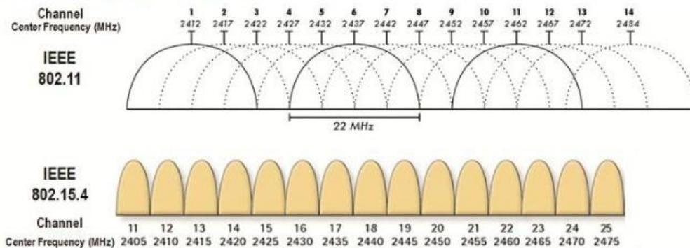
It is best to choose a channel (from 11 to 25) for Xsens communication that is not covered by WiFi use. For example, if a WiFi analyzer indicated that 50% of Channel 1 is already in use, IEEE 802.15.4 channels 11, 12, 13, or 14 would not be good to choose for Xsens communication. Typically, channels 11, 15, 20, and 25 are not used by WiFi.
