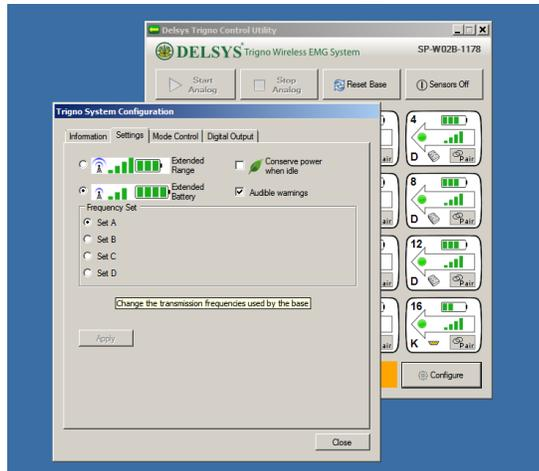
When collecting EMG data with Xsens data, the Trigno system (in any frequency setting) will affect communication over radio frequency channels 13, 20, and 25. If Xsens is using one of these three channels, there may be issues with hardware activation due to inability of all sensors to wirelessly connect to the base station. If activation is successful, dropouts in data may occur. An example of this dropout is seen below for Xsens sensors 1, 2, and 5.
