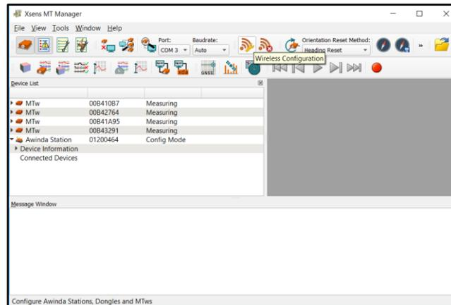
Select a channel for each Awinda device in the Wireless Masters list and click the Enable All Wireless Masters button. As the undocked sensors connect to the Wireless Masters, their signal strengths will be displayed. Selecting different wireless channels can result in different sensor signal strengths, based on potential sources of environmental interference.
