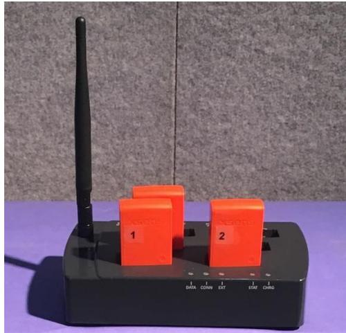
Pictured above is an Awindia Docking Station with (3) MTw Awindia 3DoF sensors. The Awindia Docking Station charges the sensors when docked.
