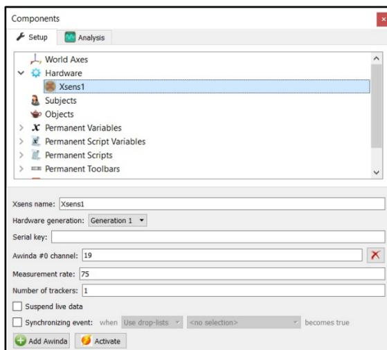
For setting the measurement rate, see the table below. The Number of trackers should match the number of MTw sensors that are being activated.
