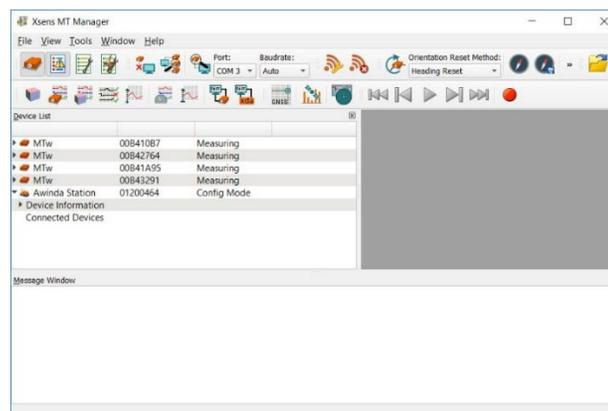
From the Tools menu, select the Power Off > All Devices menu option. Note, only devices that are connected and listed in the Device List will be powered off. If the power is cycled to a docked or otherwise connected MTw sensor after it has been powered off, it will be turned back on as described in the Powering on the sensors section.
