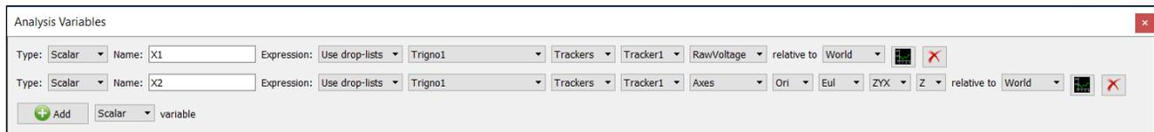
In addition to the data types available for Channel type sensors, Tracker type sensors have the option of Orientation or Acceleration data, depending on the IM tracker auxiliary data type selected in the parameters panel.
