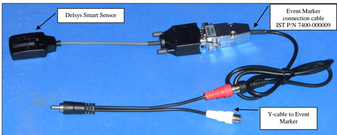
2. The Synchronizing event will be based on the channel that the Delsys Smart Sensor is attached to. In the picture above, the Smart Sensor is connected to EMG Sensor #5 so The MotionMonitor xGen settings for the Synchronizing event might be as seen in the image below.
