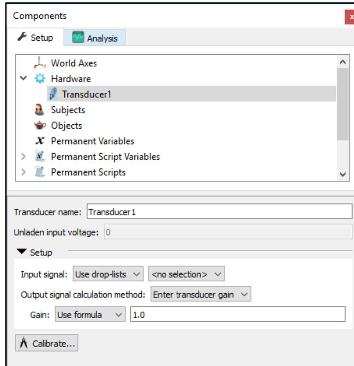
If selecting "Enter transducer gain" for the Output signal calculation method, the Gain factor can be specified either using a formula or the drop-lists. The calculation of the transducer's output would be calculated as follows:
