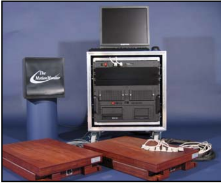
The MotionMonitor base unit shown here with Ascension magnetic trackers, Extended Range Transmitter and Bertec non-conductive forceplates.
